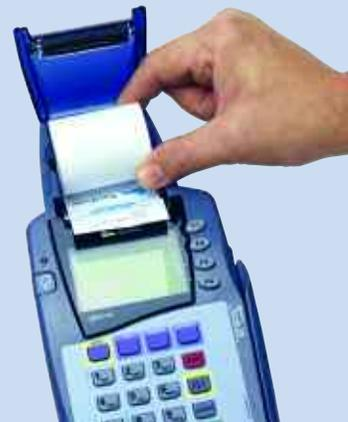
*A “clam shell” printer facilitates drop-in loading, virtually eliminating paper jams.*
